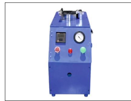
RPT UNIT (vacuum For Porosity Measurement)
